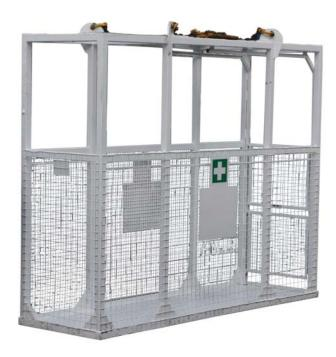
Designed as a safe method of transporting injured personnel with an attendant, from any structure or excavation. Especially useful in any situation where the only alternative is for a stretcher to be manhandled up or down ladders or stairs. The CA121 comes complete with a four leg chain set attached to the main lifting lugs with couplers. This chain set is rated to give a ratio of 10: 1 as required by the CE regulations.
