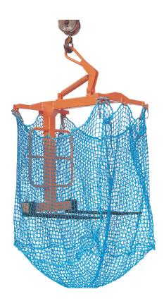
The 1056 has been designed to give flexibility when required to move oversized and normal packs of block and brick s as well as palletised goods around site. This unit is supplied with heavy duty sprung lifting eye allowing automatic levelling of any load being carried. The unit also comes supplied with net hooks allowing the addition of a load safety net
