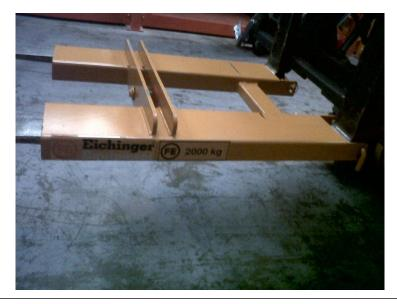
The fork mounted load hook enables the conversion of any fork lift unit into a simple mobile crane unit allowing the lifting of items by chains and slings in a secure and safe manner. As with all Eichinger fork mounted units the 2084 is secured to the fork lift by a heel pin NOT chain. Always use the load hook in relation to the load capacity of the fork lift truck!
