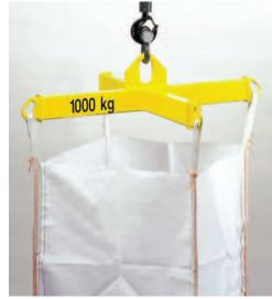
The TTB big bag lifters are designed to lift and transport large bags safely and securely. They are manufactured as a 4 point spreader beam in a fixed frame. The construction incorporates 4 hooks with safety latches that allow fast loading and unloading of the bags.
