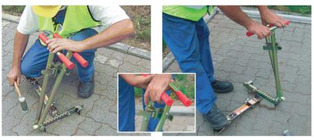
The profiled spring steel blades of the new Probst paving block extractor SZ are driven into the joints with the combination hammer KH (steel side) and jammed. The gripping force is held without physical effort by means of the locking device. This locking device does not need to be used on new installations when the joints have not been filled with sand and the pavers can be extracted quickly.
