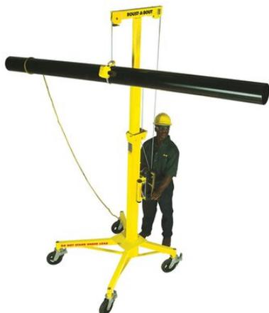
Roust-a-bouts are capable of lifting up to 680kg and to a height of 7.6m (25ft).
