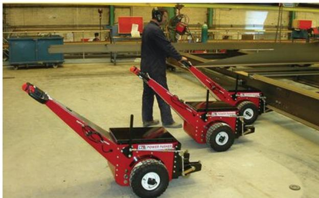
The Power Pusher is a versatile pedestrian-operated, electric tug/utility vehicle used to move, push, pull, steer and manoeuvre industrial loads.
