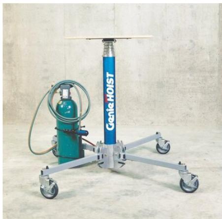
This pneumatic hoist is powered by either CO2 or compressed air and makes easy work of positioning loads such as ductwork or ceiling panels in restricted areas. Its compact design allows it to be folded up and fitted into the boot of most cars. [... Read more](#)
