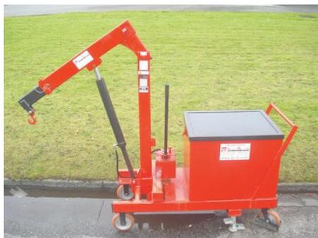
Manoeuvrable floor crane providing an overhead lifting point where no lifting point exists.
