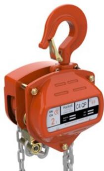
The William Hackett C4 QP chain hoist incorporates the four-pawl mechanical engagement functionality. The unique and patented pawl design enhances the capabilities of the hoist allowing all four pawls to engage with the ratchet gear in an offset configuration allowing finer adjustment and tensioning capability while maintaining pawl/ratchet engagement. This improves the hoist's -
