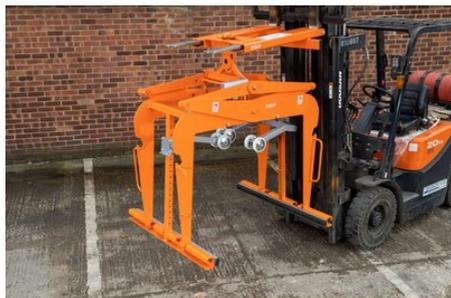
Designed to lift, move and release numerous types of slabs, blocks and single or double layer kerb packs safely on a building site or yard, up to 1800kg. Fully mechanically operated via the forklift (without the driver leaving the safety of his seat) or via an overhead crane / HIAB.
