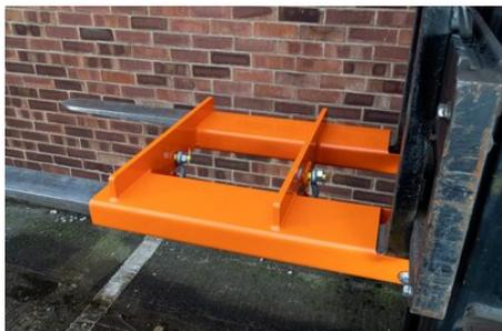
Fork Mounted Hook Fork Mounted Hooks provide an economical and safe method of converting a forklift into a mini mobile crane. Multiple lifting positions can be achieved along the fork blade.
