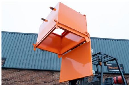
Bottom Empty Skip of light to medium weight waste when being automatically emptied into high sided yard skips via the base release mechanism, without the driver leaving the safety of his seat.
