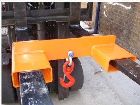
The Adjustable Fork Mounted Hook provides a quick and economical method of the lifting and positioning of unpalletised loads. Multiple lifting positions can be achieved by the correct positioning of the attachment along the fork blade. This compact unit has been designed for when space is at a premium storage, transportation and the actual fit.
