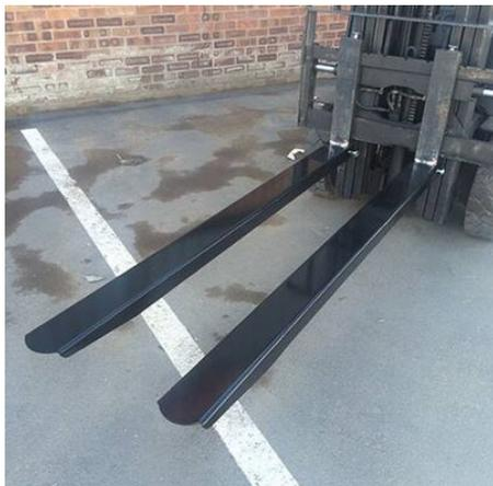
Fork Extensions provide a simple, but effective method of handling the occasional long and awkward load that extends past the tips of the parent fork arm (maximum overhang 66%).
